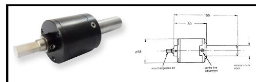
This head is designed primarily for producing hexagonal holes. A micro screw is provided to set the cutting bit on the machine centre line. The inner shaft is mounted on sealed ball races for precision and long life.
